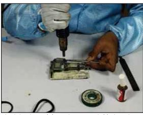
Fig: 3.2.5.8 Headphone Connector Soldering - Step 1
