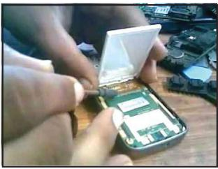
Fig: 3.2.5.16 Display Strip Assembly
