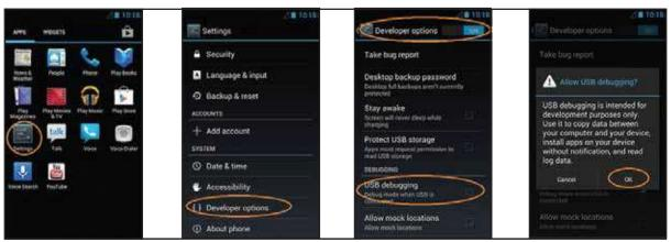
Fig: 2.4.12.2 USB Debugging Mode -Android 3.0 - 4.1 X
