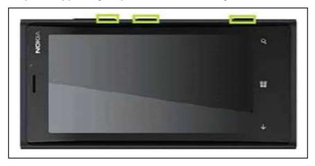
Step 3: Press the Volume Down Key + Power Key to turn on the unit
