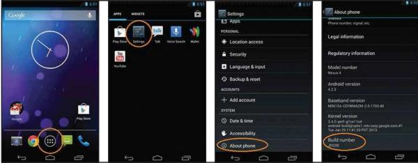
Fig: 2.4.12.3 USB Debugging Mode -Android 4.2
