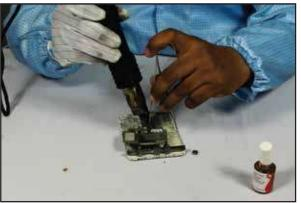
Fig: 3.2.5.4 Charging Connector Soldering - Step 1
