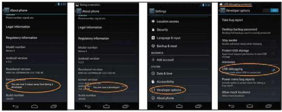
Fig: 2.4.12.4 USB Debugging Mode -Android 3.0 - 4.1 X
