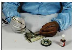
Fig: 3.2.5.5 Charging Connector Soldering - Step 2
