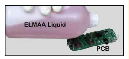
In such case we need to do the servicing of the mobile. We have to use Elmaa and IP liquid used to wash the PCB. First we need to remove all metal cover and then start washing the PCB.
