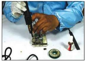
Fig: 3.2.5.9 Headphone Connector Soldering - Step 2
