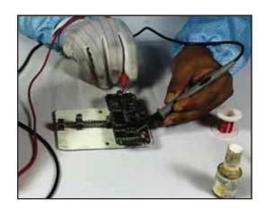
connection will be made through jumpering. Exactly the same way we need to give connection from this point to that point and again for this point to that point we need to do the jumepring for connectivity. This is the solution we can do if even after replacing headphone connecter left side or right side is not working.
